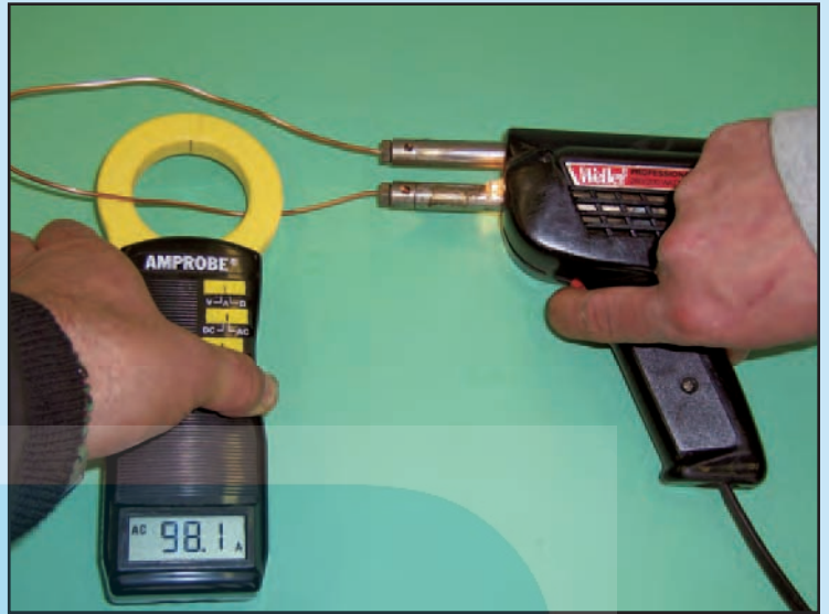
Color Plate 15: When a #12 AWG wire is loaded at 100 amps by the high-current transformer in this soldering gun (even momentarily), it heats up very quickly, as you can see. At 98.1 amps, the wire starts to turn color from the heat after only a few seconds. Chapter 16 provides more information about calculating current loads for branch circuits.
